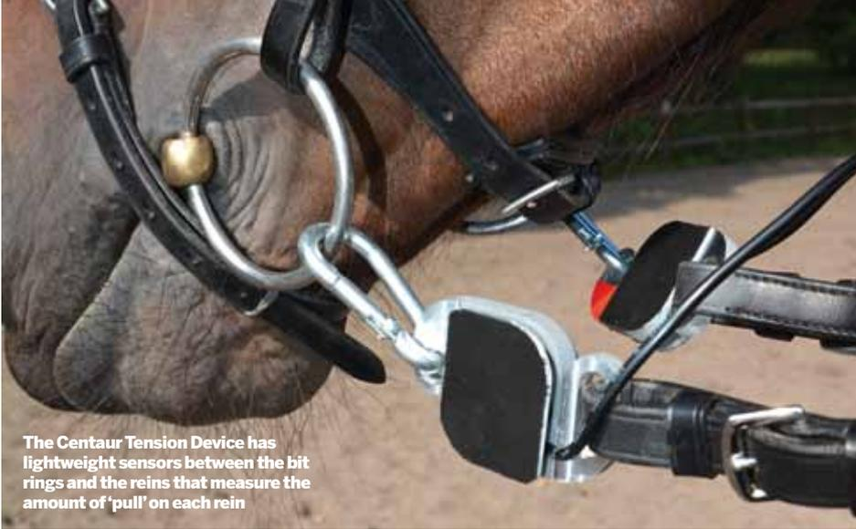
The Centaur Tension Device has lightweight sensors between the bit rings and the reins that measure the amount of 'pull' on each rein
